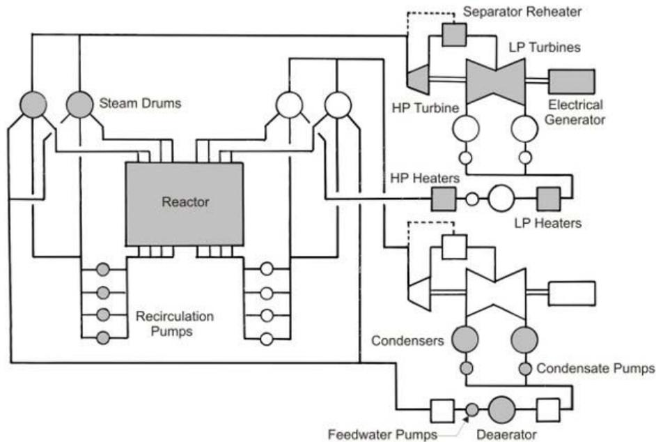
Figure 6: Reactor coolant and steam supply circuit
