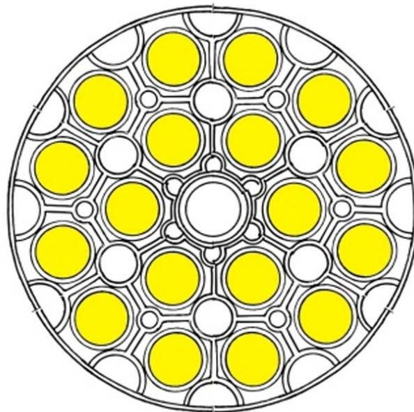
Figure 5: Fuel bundle showing supporting grid
