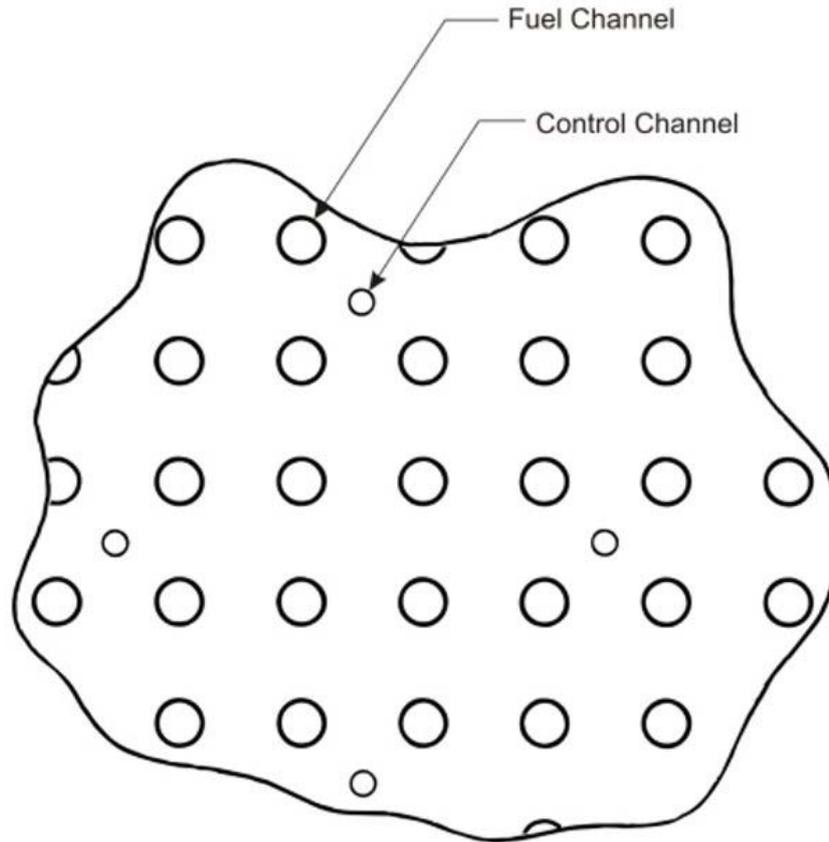
Figure 2: Reactor core part cross section
