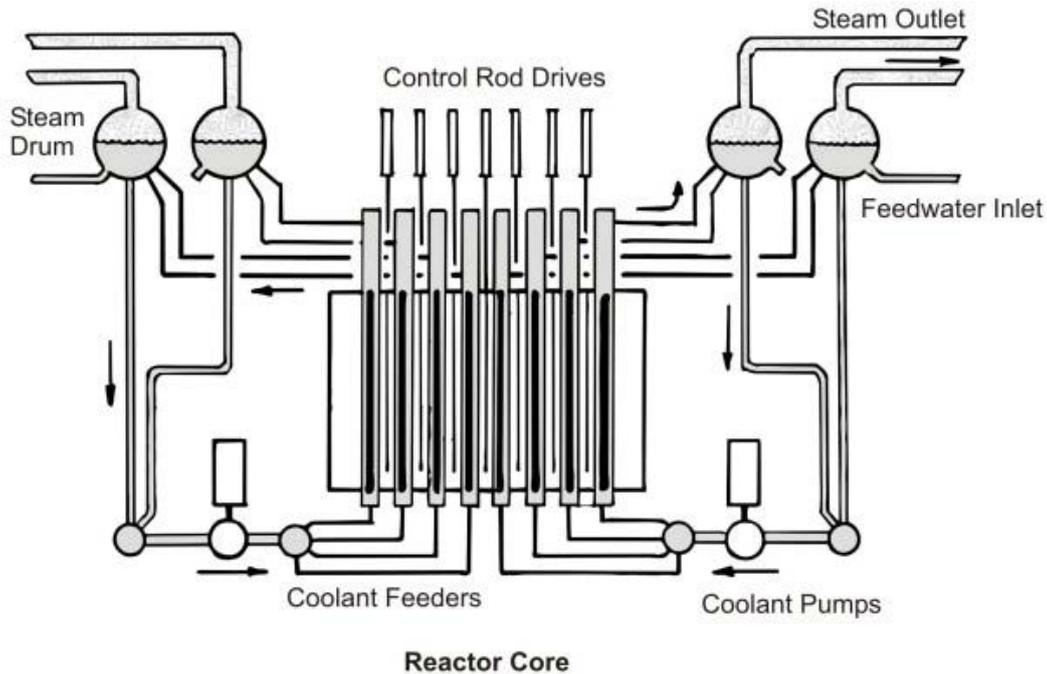
Figure 1: General arrangement of reactor
